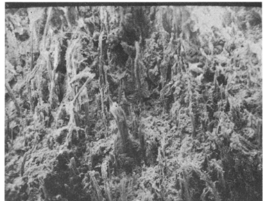
Figure 15 A typical SEM fracture surface of an asbestos cement ( m_f = 0.15 ) showing the predominant fibre pull-out mechanism ( \times 35 ).
